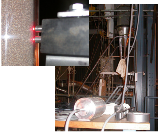
Fig. 3: Labasys® 100 Flex instrument at a pilot plant (right) and tip of the instrument (left).
