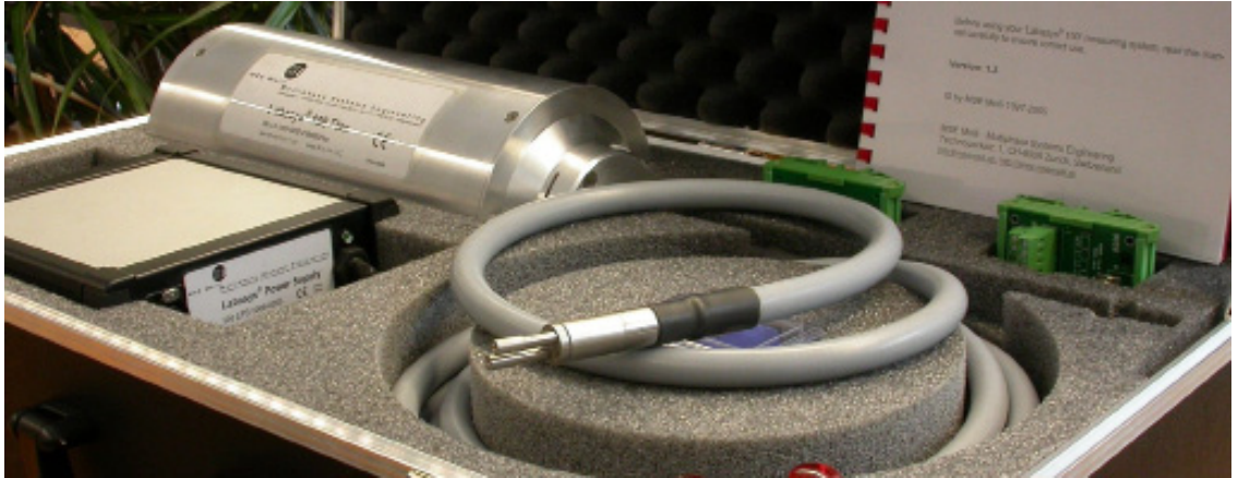
Fig. 2: Labasys® 100 Flex instrument for velocity measurement of bulk solids with 6 m flexible tip.
